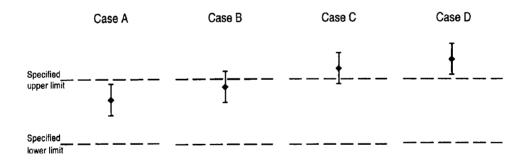
J2.2 In Case A, the reported value (indicated by ♦), extended by the uncertainty of measurement, lies within the specification limits. A statement of compliance can therefore be made for the confidence level stated.
