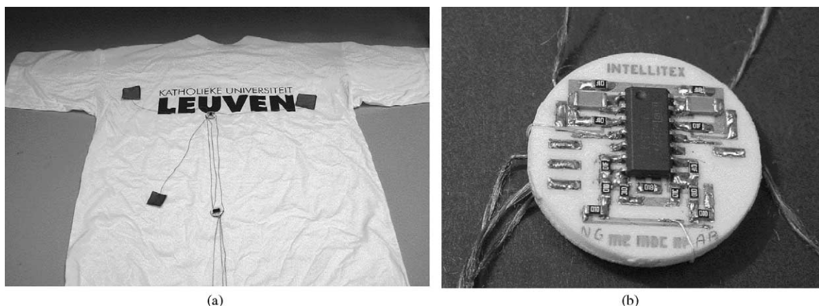
Fig. 15. (a) Concept of the integration: distributed network with stainless steel yarn bus system. (b) Detail of the ECG read-out circuit button.
