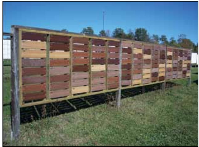
Figure 11–17. Extruded wood–thermoplastic composites being evaluated for a siding application (Clemons and Stark 2007).
