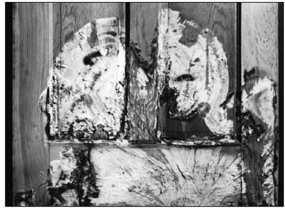
Figure 14-4. Mycelial fans on a wood door.
