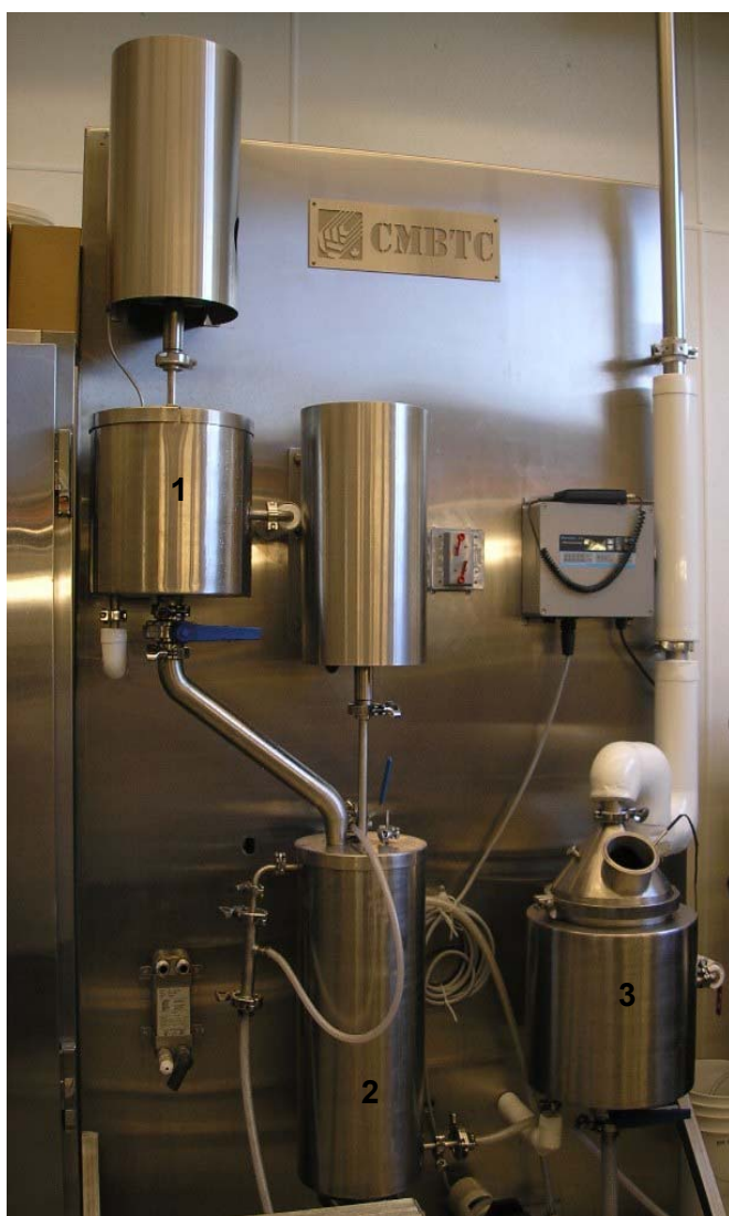
Figure 3.2 Micro-brewing at the CMBTC. 1: mash mixer; 2: lauter container; 3: kettle (boiling) (By Blanca Gómez G).
