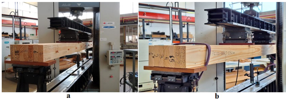
Figure 3. Test set up for bending tests. a. DLT panel. b. WNLT panel.
