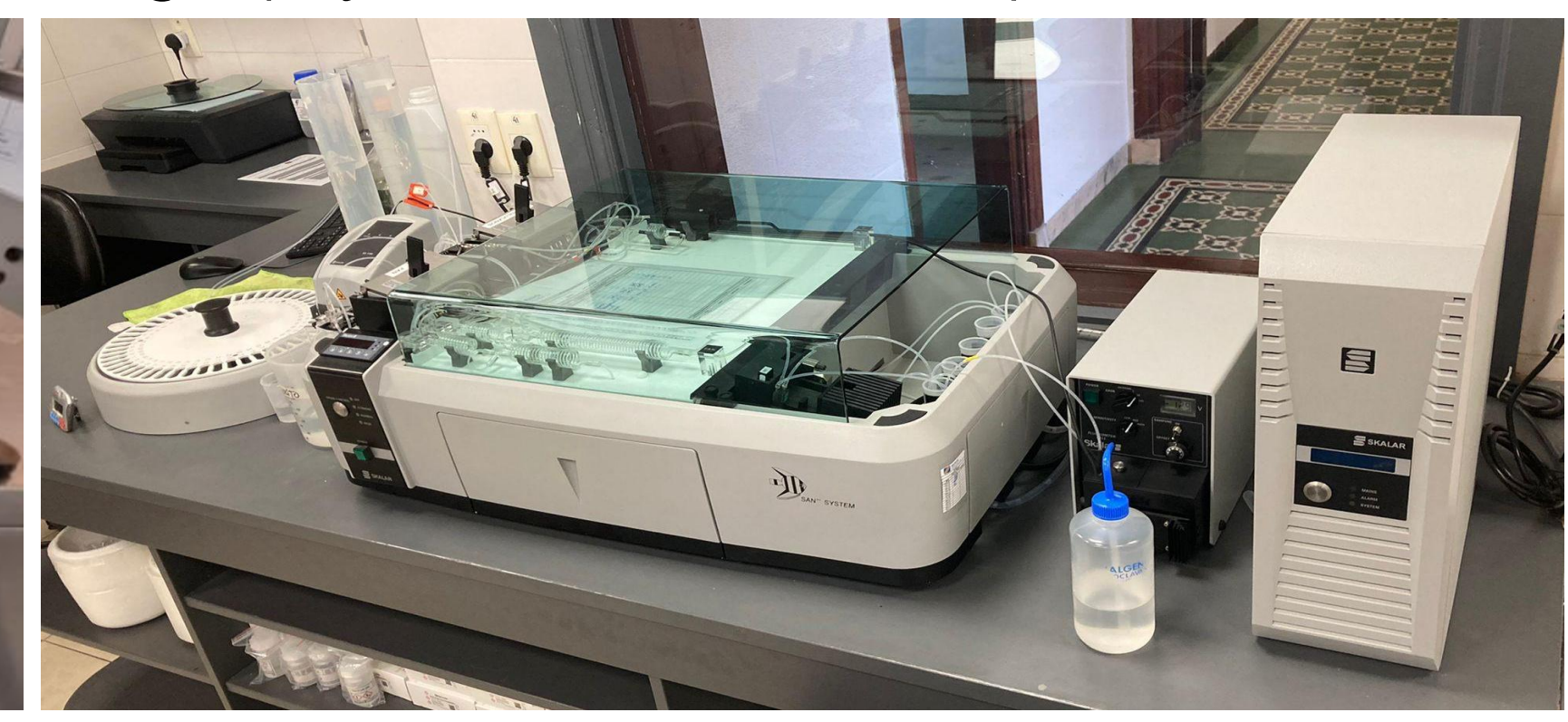
Figure 3. Skalar model SAN++ equipment (with module to measure BG, sampler SA1000, fluorometer SA6310) in Maltería Oriental S.A.
