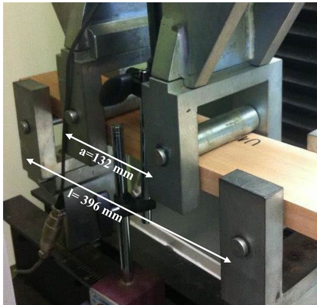
Fig. 2 4-point bending tests of the finger-joint in the universal bending machine Minebea
