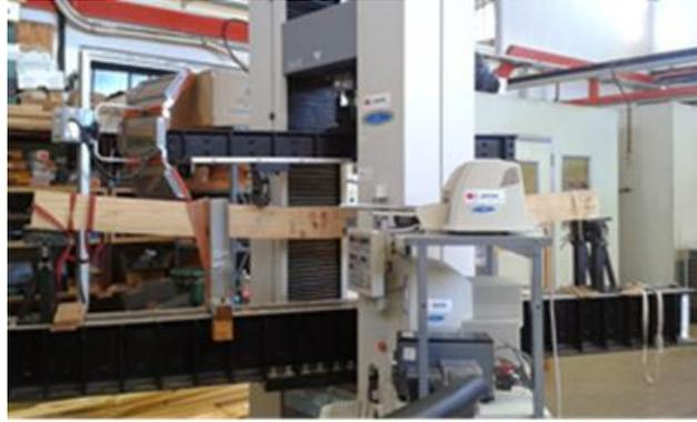
**Fig. 3.** Static four-point bending test set up
