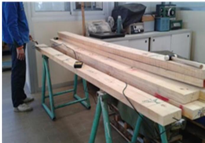
Fig. 2. Dynamic NDT set up
