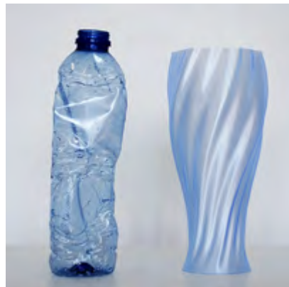
3d print made from Refil PET from old bottles
