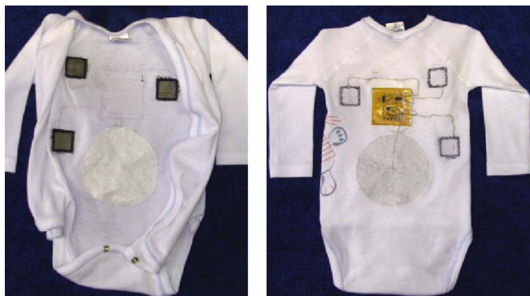
Fig. 8. Baby suit prototype. Left: inside showing the Textrodes; right: backside.
